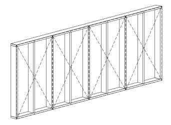
NB: Creating another similar wall-panel and then nailing the ends of two panels together at 90 degs to each other ~ with the meeting ends (vertical edges) flush with each other ~ will automatically guarantee that a truly vertical corner is created every time!
